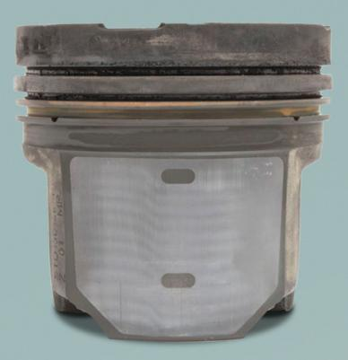
These parts were pulled from a 2014 PACCAR MX-13 pulling a refrigerated trailer in coast-tocoast service from its base in the southeastern US. Oil drains were at 45,000 mile intervals using Guardol FE<sup>®</sup> 10W-30 (FA-4). Tear down was performed in 2017 after quickly accumulating 500,000 miles.
